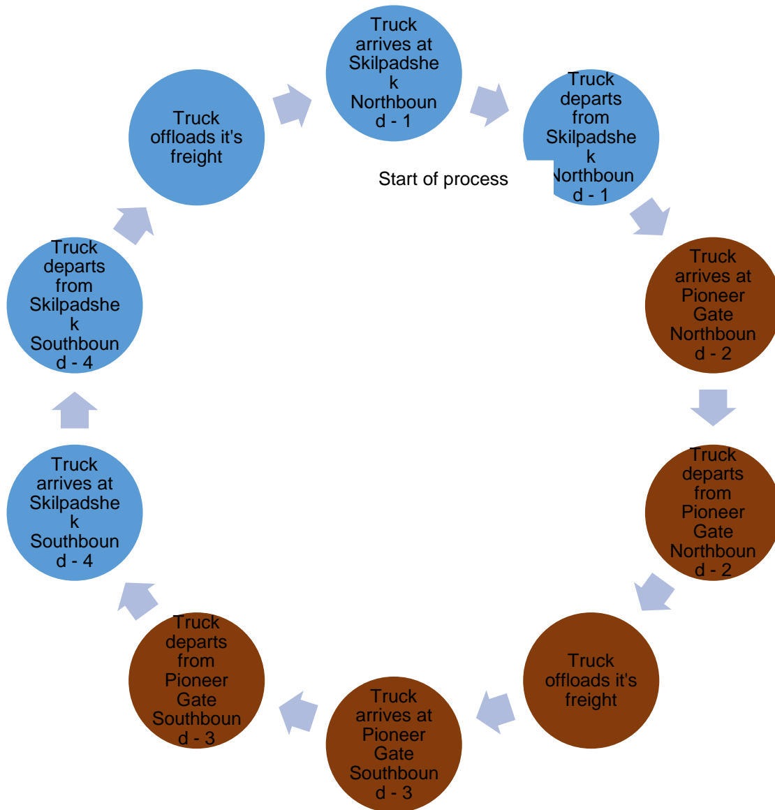
Figure 10: Border process of truck time recordings for valid entries
